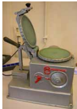
Figure 3. 2: automatic mill provided by Old Holland for the preparation of reconstructed oil films
