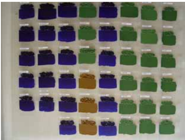
Figure 3. 1: reconstruction paints using ultramarine, chromium oxide green and raw sienna and variable amounts of drying oils and additives
