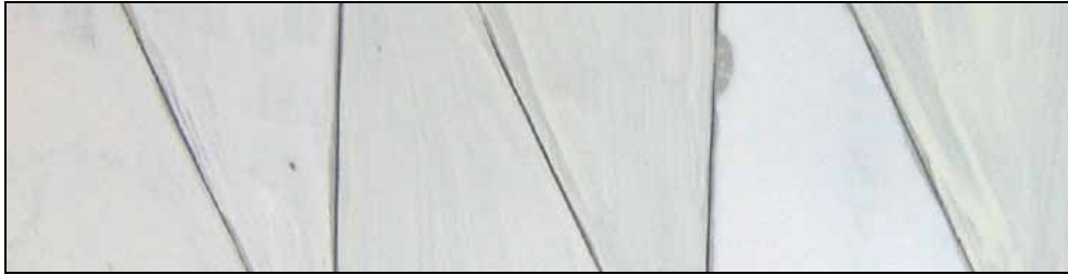
Figure 4. 4: ZnO in cold-pressed linseed oil and in stand oil; 2PbCO_3 \cdot Pb(OH)_2 in cold-pressed linseed oil and in stand oil; TiO_2 in stand oil and in cold-pressed linseed oil (from left), 2008
