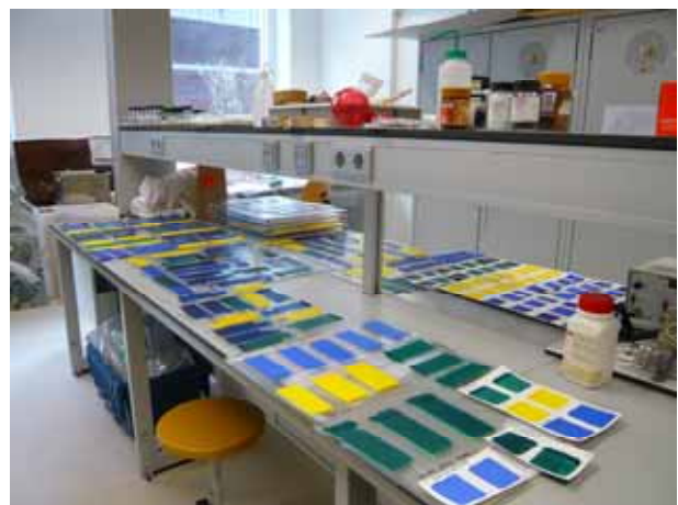
Figure 3.12: Laboratory-prepared samples from modern tube oil paints (W&N, Talens and Old Holland)
